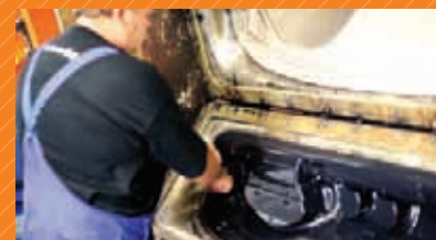
DASH-BOARD SKIN PEELED OFF FROM SLUSH-MOULDING TOOL
