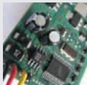
LIN-bus-systems in exterior mirrors (Jaguar)
