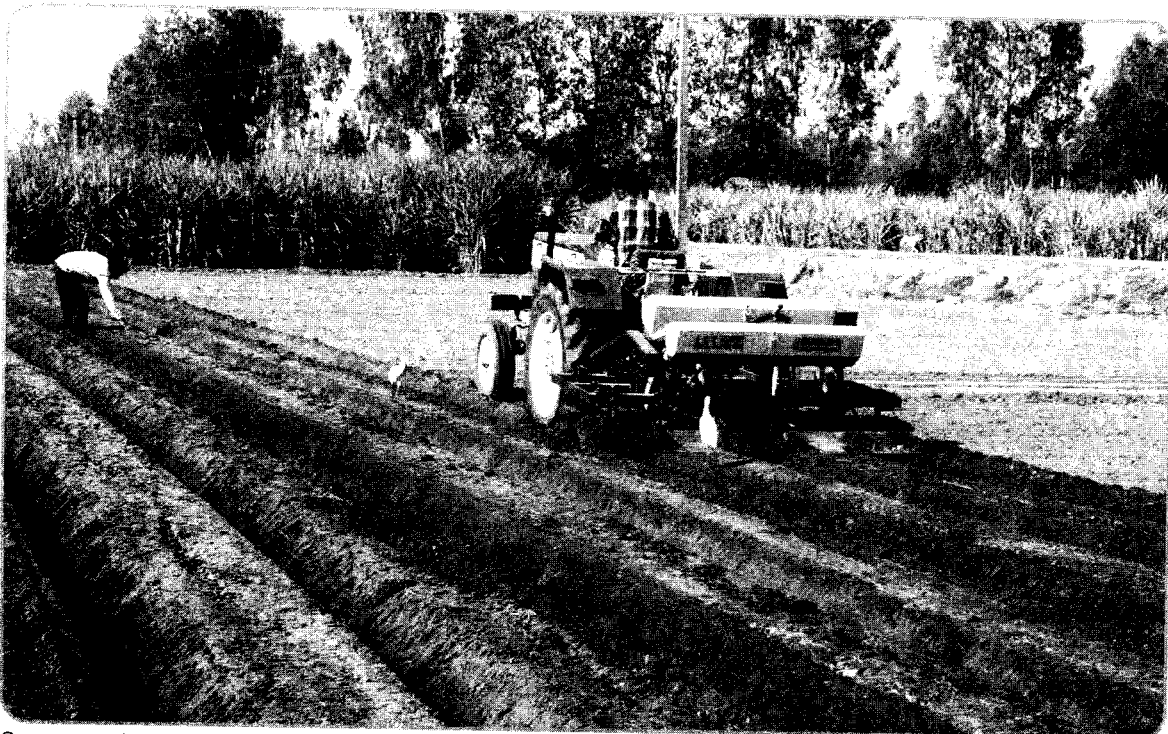
Sugarcane planter preparing raised beds for growing wheat as an inter-crop with sugarcane.
