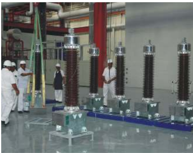
State-of-the-art facility at Hosur manufactures CVTs ranging from 72.5kV to 1200 kV
