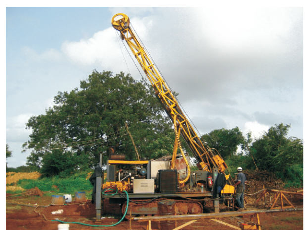
Fig-3 : Diamond Core Drilling operation at Ganajur Main Gold Prospect, Ganajur-Karajgi PL.
