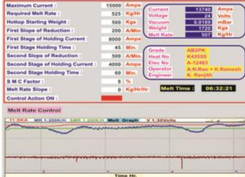
Modernised With In House Developed PLC Control Automatic Process Controller Data Logging System
