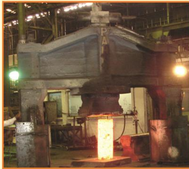
Re-vamped 1500 MT Forge Press brought into operation
