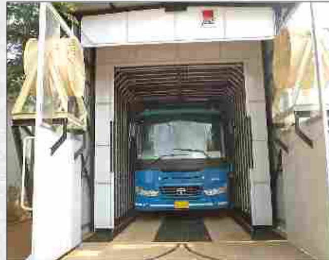
Shower Test Facility for buses
