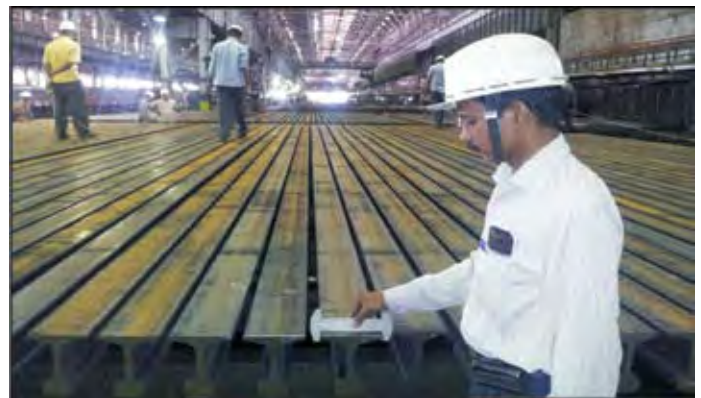
Third Party Inspection of rails at Bhilai Steel Plant
