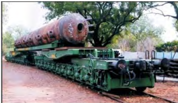
Design of 24-Axle 300t Special Wagon for BHEL, Tiruchirappalli
