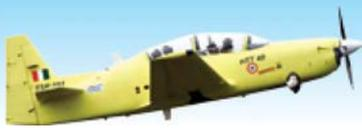
financed project. Towards flight trials and certification activities, first Prototype of HTT-40 was rolled out on 29th January, 2016, 37 Nos of Engine Ground Run (EGR) completed and Low Speed Taxi Trials (LSTT) were commenced in March, 2016.
