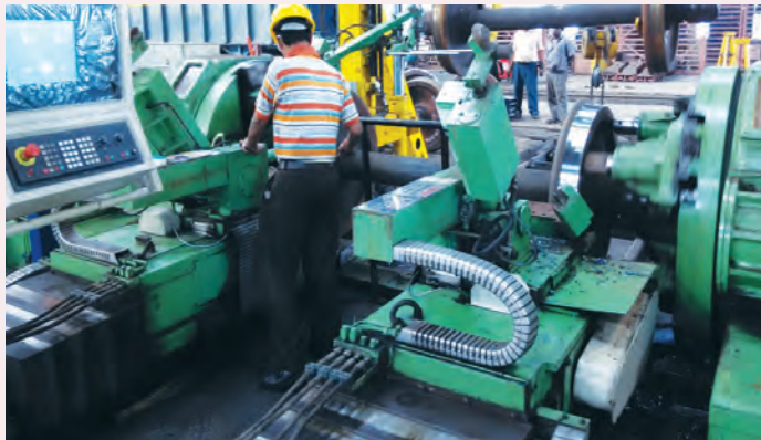
Wheel reprofiling on wheel lathe
