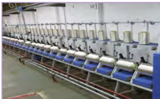
Indigenously developed Zero-twist rewinding machine
