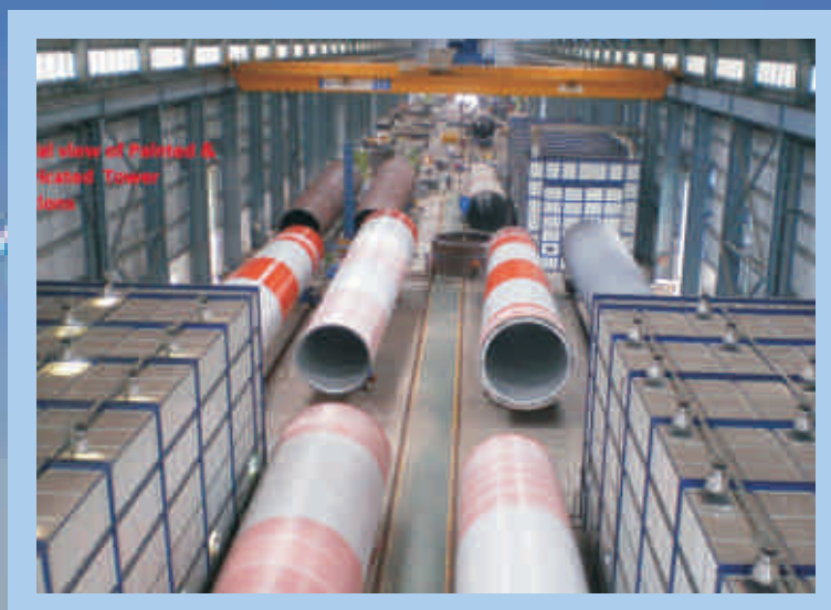
Painted & Fabricated Tower Sections
