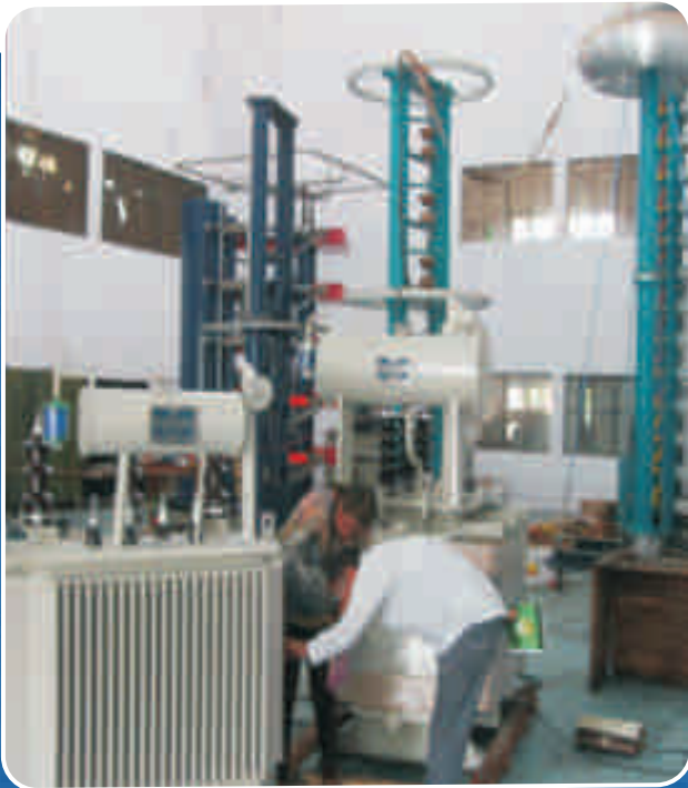
Impulse test of Distribution Transformers at National Test House Ghaziabad witnessed by EEPCO Ethiopia engineers
