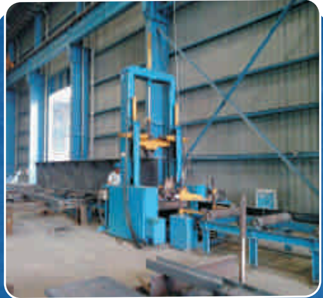
Automation through tech-welding Machine in fit up section
