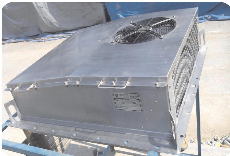
Driver cab AC Designed and Developed for Diesel Locomotive
