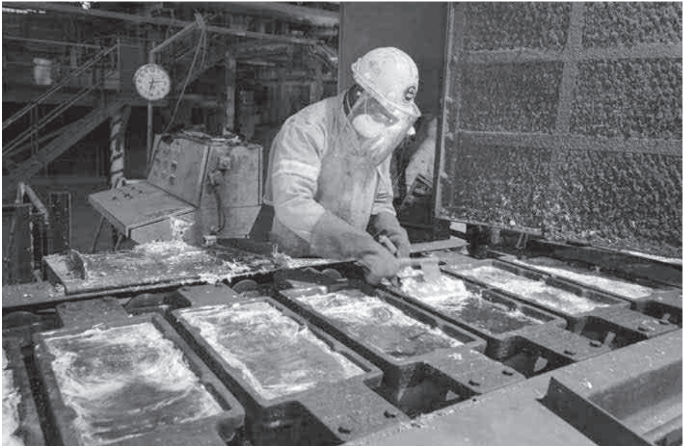
Skimming of final metal ingot production
