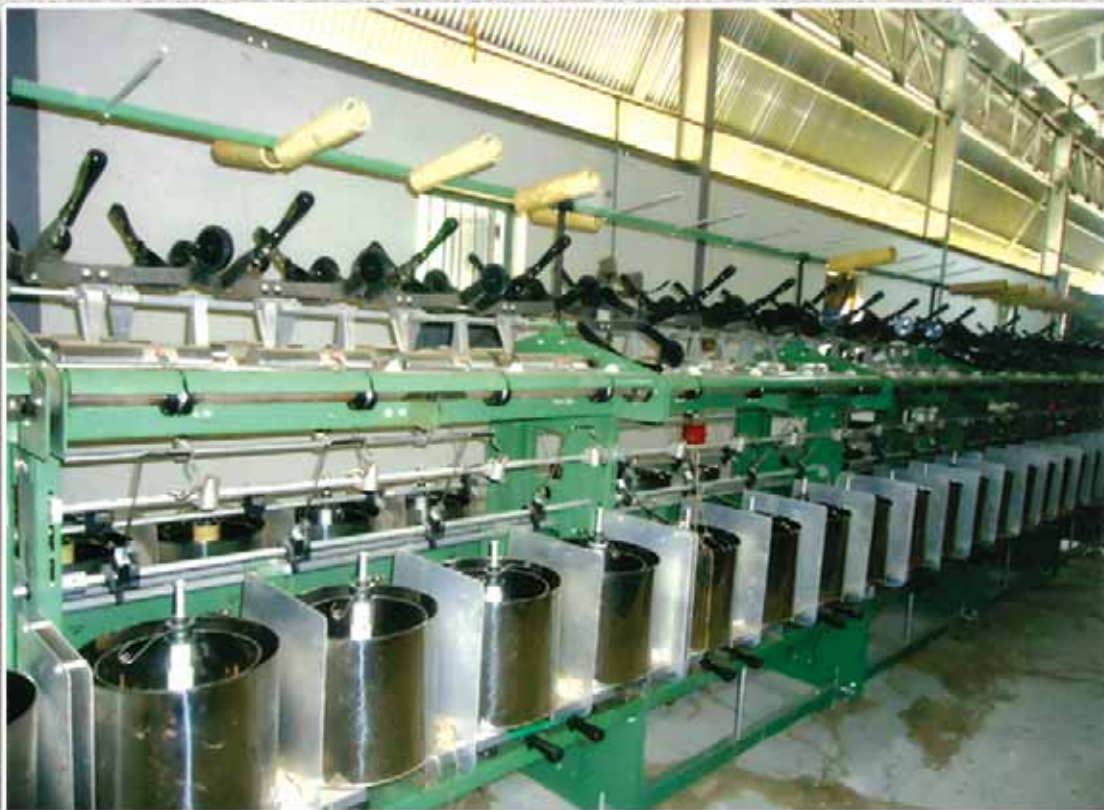
The TFO (Two-For-One) Twisting Machine at Birla Jute Mills, Birlapur, West Bengal
