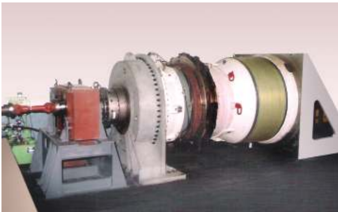
◀ 1MW wind turbine planetary gearbox on factory test bed.
