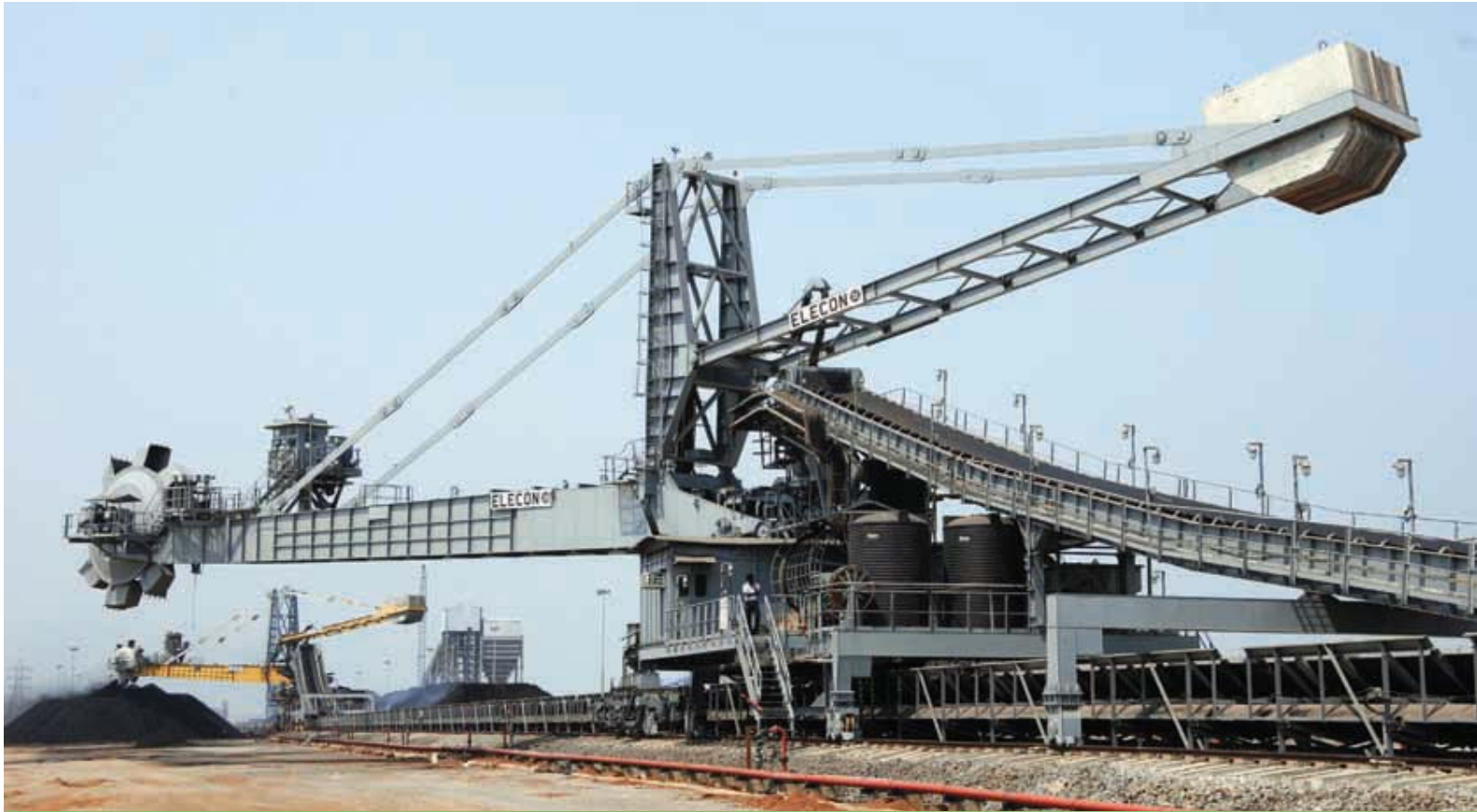
Bucket wheel Stacker cum Reclaimer handling Coal at Chetnad Port having stacking capacity - 3850 MTPH and Reclaiming capacity - 2400MTPH.
