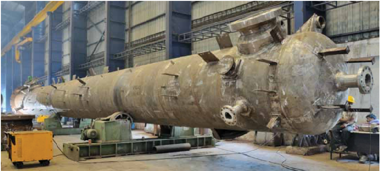
RCF - THAL - (SS 304L) CONDENSATE STRIPPER COLUMN
