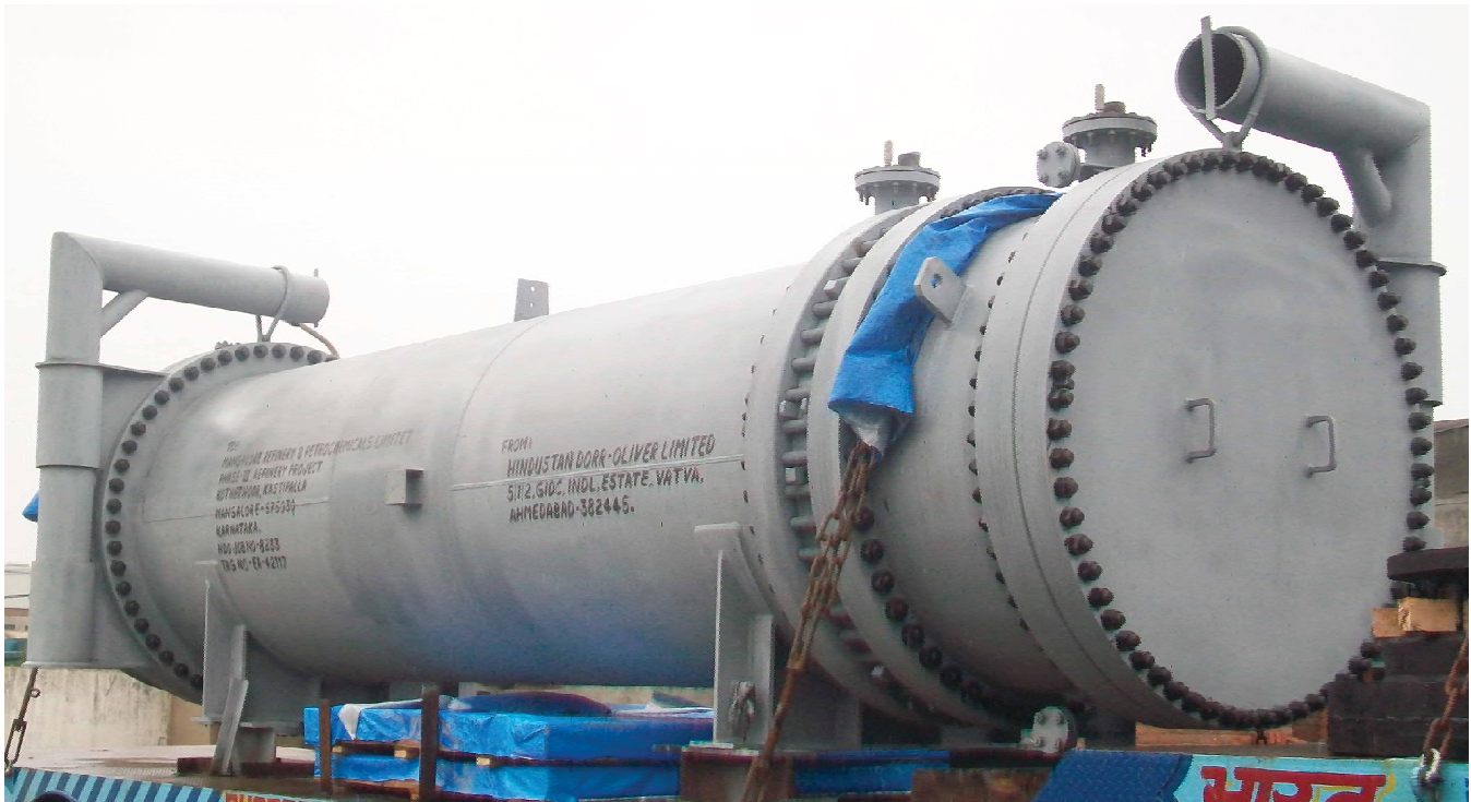
MRPL REFINER - STORAGE AFTER COOLER
