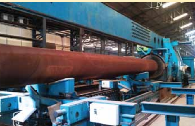
High Pressure Hydrotesting at Pipe Mill in Progress
