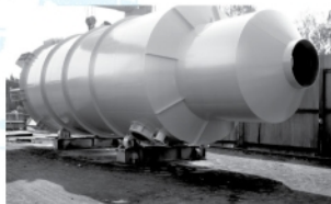
Petrofab Division (Vadodara Works) Fabrication of Oleum Tower for Bodal Chemicals Pvt. Ltd.
