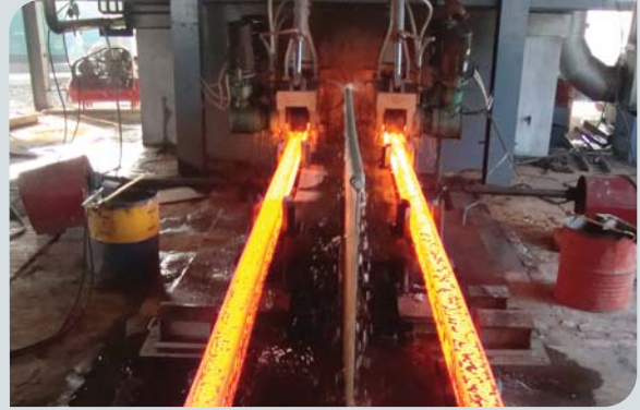
Continuous Casting Plant at Bihta
