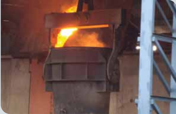
15 Tonne Capacity Ladle carrying molten material to CCP
