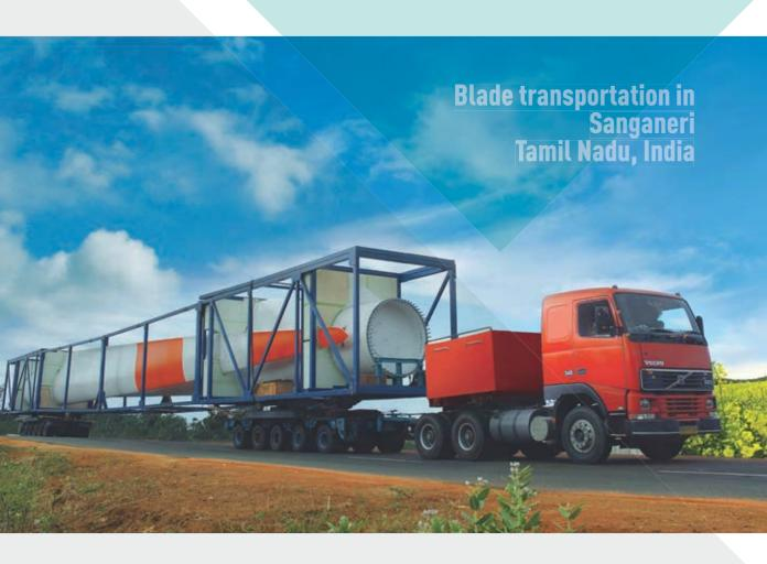
the blade has been challenging due to constrained road conditions. The logistics team at Suzlon developed an innovative two fold transport system, which used a specialised 'Adapter Trailer' for the first time in India. This innovative approach ensured unbound manoeuvrability through the hilly terrain, while transporting long blades safely in a cost-effective and time-efficient manner to the most remote wind sites.
