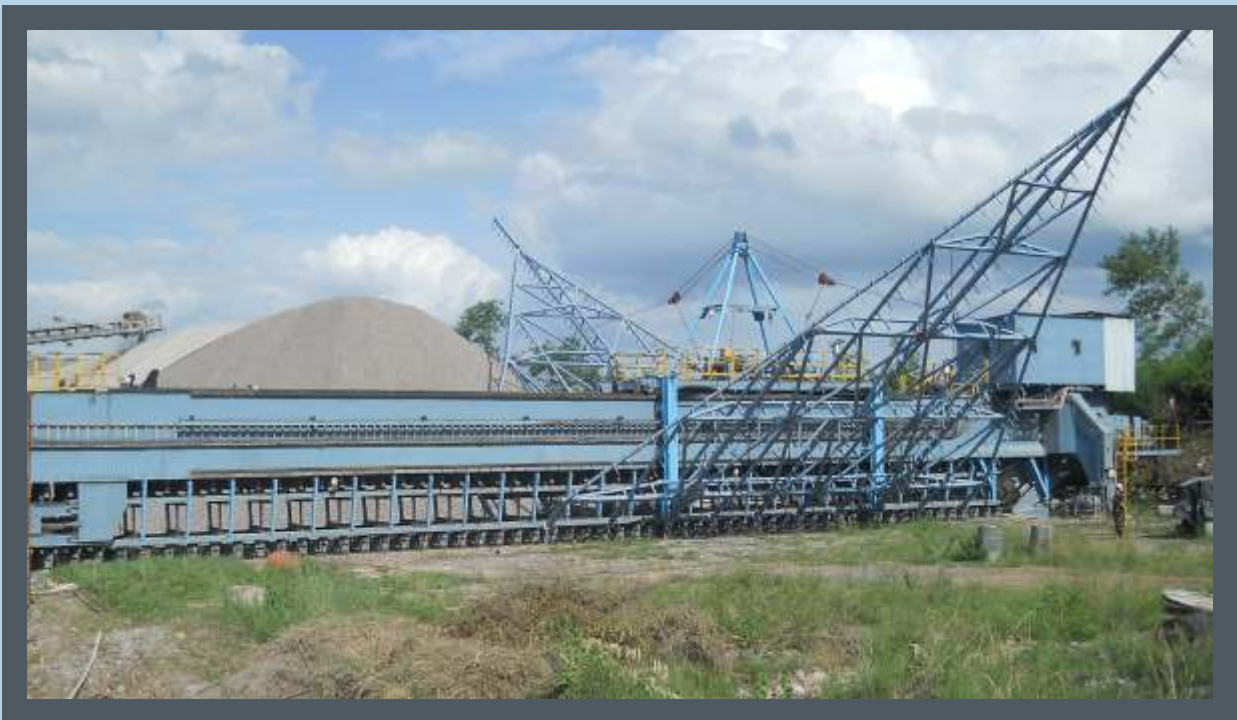
Bridge Reclaimer manufactured, supplied & commissioned for limestone handling for Orient Cement, Andhra Pradesh. This has a capacity of 1000TPH with rail CRS of 40m.
