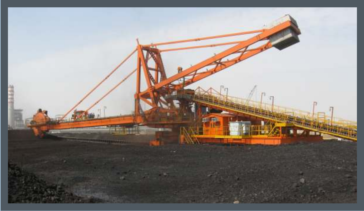
This Bucket Wheel Stacker cum Reclaimer designed & manufactured by Tecpro for 8 x 135 MW Rajwest Power has a capacity of 1200 TPH while stacking and 1200 TPH while reclaiming with boom length of 35m.
