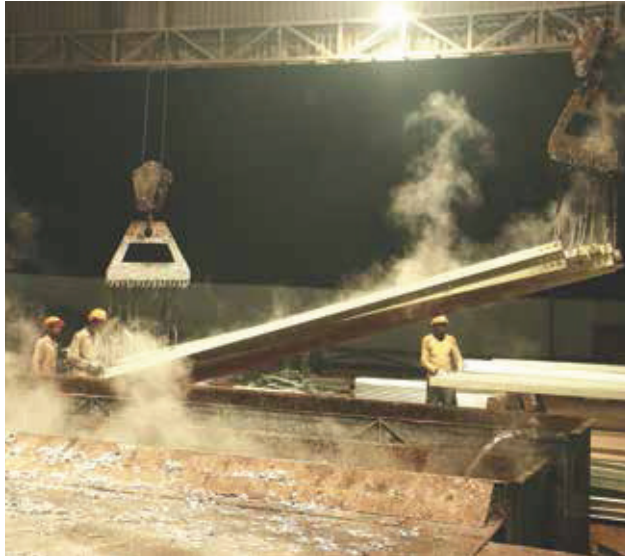
▶ Galvanising process at our tower manufacturing facility
