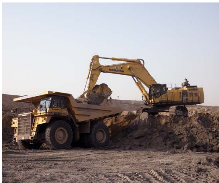
Komatsu PC1250 Hydraulic Excavator loading Komatsu HD785 Dump Truck in opencast project
