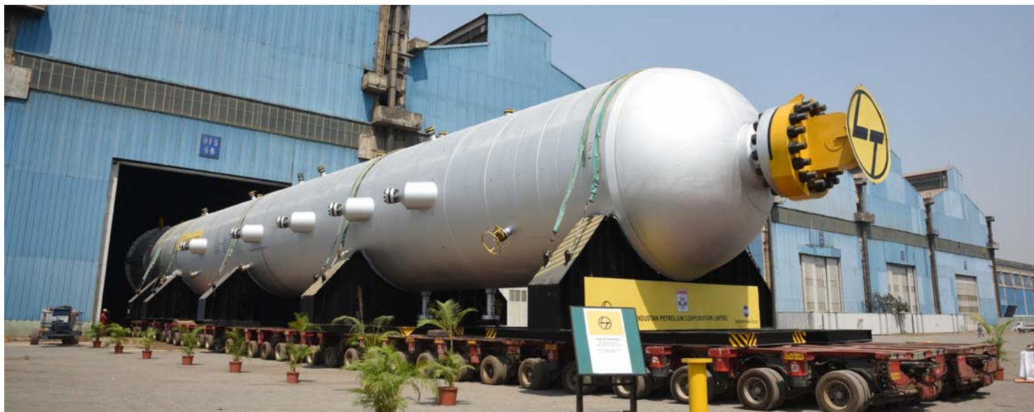
India's heaviest Hydrocracking Reactor (1858 MT) for HPCL Visakh Refinery
