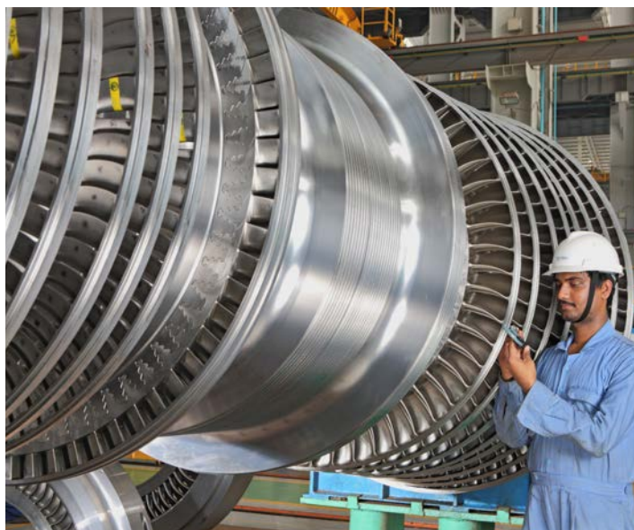
Supercritical turbine being manufactured at Hazira, Gujarat
