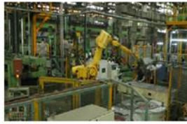
Gravity die casting cell
