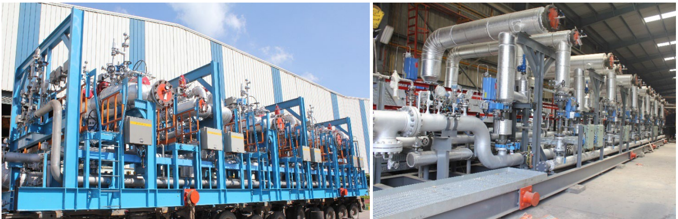
Process for Manufacturing Modular Piping (Skids and Modules)
