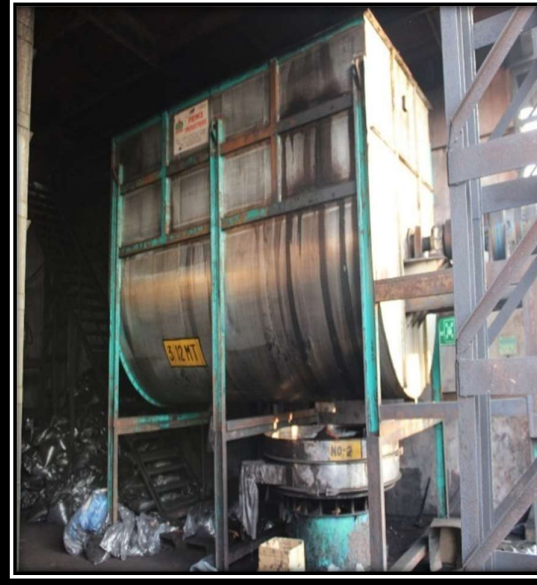
Machinery Name: 12mt Blender Location In Plant: Blender Area Capacity: 12000KGS Use: Blending Material
