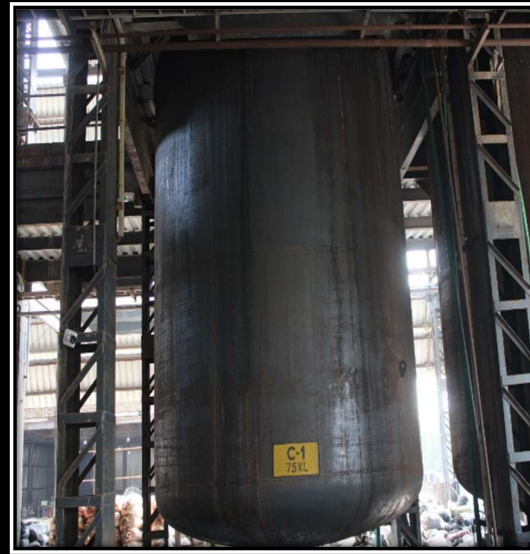
Machinery Name: C1 75KL Location In Plant: Main Plant Capacity: 75000LTR
