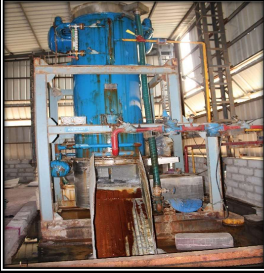
Machinery Name: Ice Flacker Machine MOTOR Location In Plant: Main Plant Capacity: 120HP
