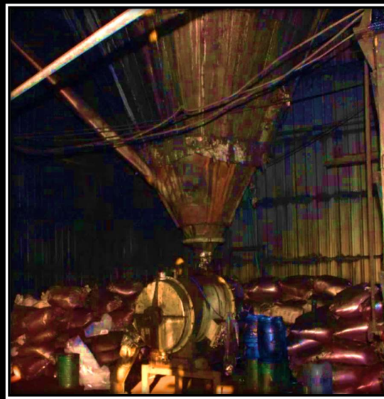
Machinery Name: Spray Dryer Location In Plant: Spray Dryer Area Capacity: 2000 Ltr Water Evoprate / Hour Use: Spray Chamber
