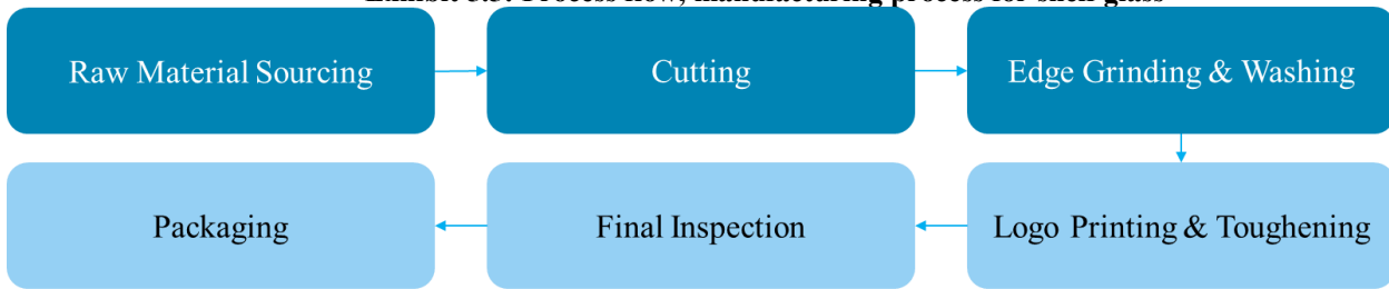
Exhibit 5.5: Process flow, manufacturing process for shelf glass
