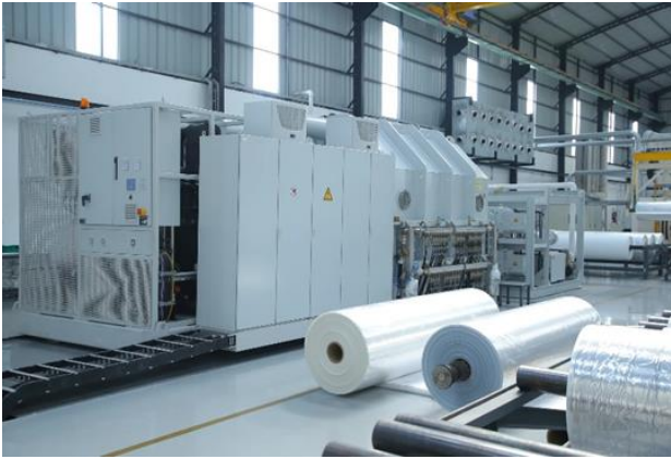
2500 mm Metallizing Machine (Buhler Germany)
