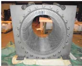
LARGER STATOR CORE - FOR SULPHARISATION PLANT. 16MW, SIZE 1500MM X 1500MM X 1700 LEN. MAX. WEIGHT = 9TON.
