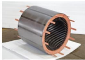
MACHINED TRACTION MOTOR STATOR CORE FOR METRO RAIL
