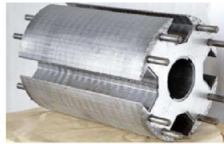
ASSEMBLED ROTOR CORE FOR ALTERNATORS USED IN DATA CENTERS
