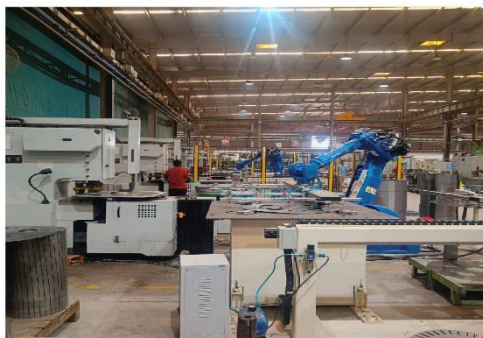
ROBOTIC LOADING AND UN-LOADING FOR LAMINATION MANUFACTURING
