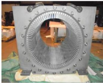
LARGER STATOR CORE - FOR SULPHURISATION PLANT. 16MW, SIZE 1500MM X 1500MM X 1700 LEN. MAX. WEIGHT = 9TON.
