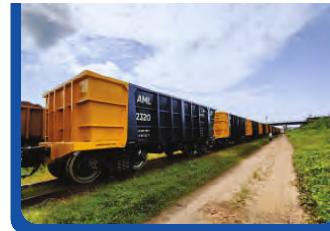
Texmaco designed and manufactured Gondola Wagon Africa, for carrying Iron Ore
