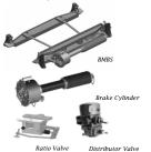
Bogie-mounted brake system
