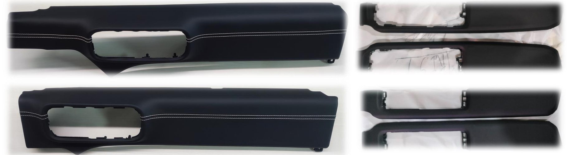
Two Stage Soft Covering Process with Hot Press Lamination
