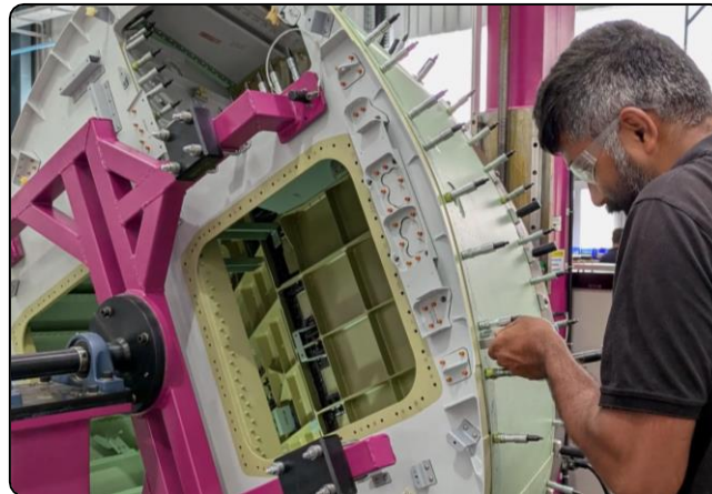
Falcon 6X Rear Fuel Tank Assembly Line
