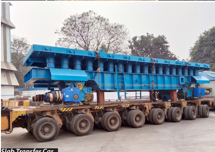
Slab Transfer Car
