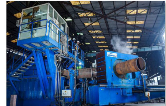
Induction bending process
