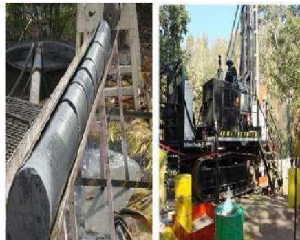
Large Diameter Kimberlite core (8") for Rio Tinto at Bunder, MP - Drilled by BLY LF230 upto a depth of 352 Meters. Largest coring done in India till date
