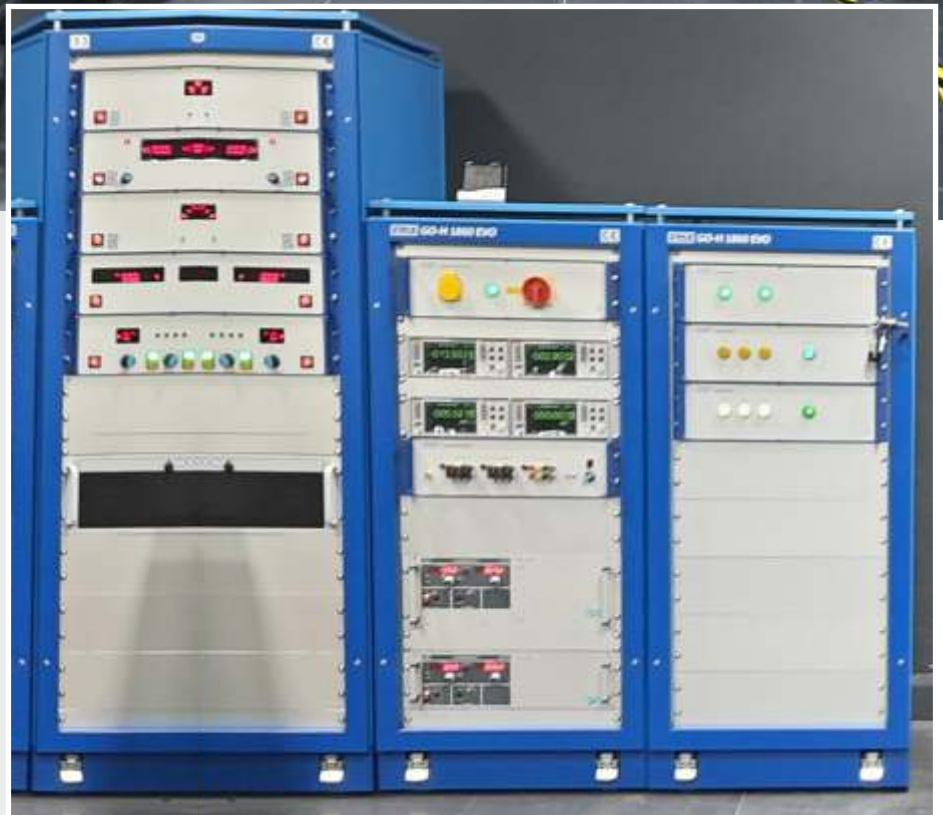
Fully Equipped Photometric Lab with LMT Germany Goniophotometer
