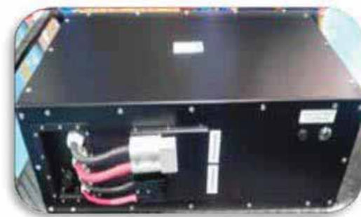
Golf Cart Battery Pack
