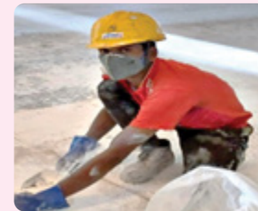
Collection of powder in bags & use as appropriate in selected batches after sieving
