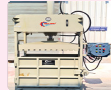
Bale press compacting for RM bags
