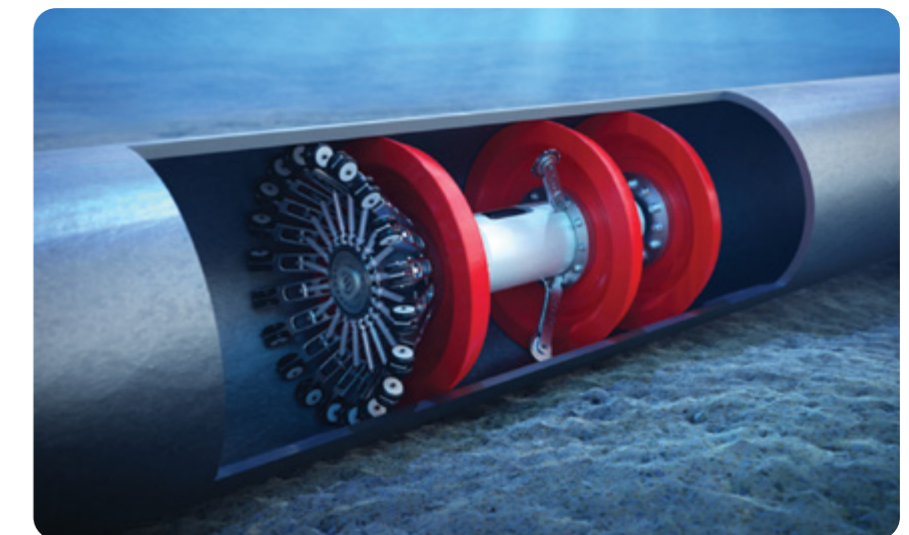
Pigging for proper cleaning of transfer lines is employed
