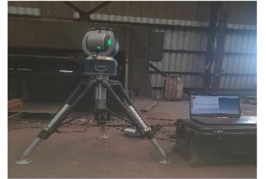
Laser tracker measuring device (Faro vantage)
