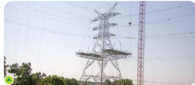
KPIL Twin Tower Testing facility in Gandhinagar, capable of testing up to 1,200 kV
