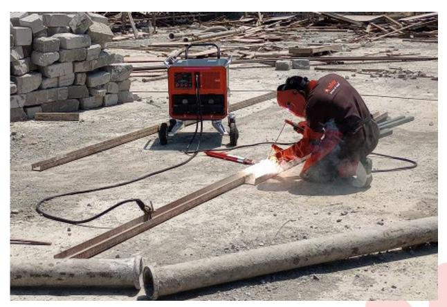
THIS BATTERY POWERED WELDING MACHINE IS BEING USED ALONG WITH ARC SENSING MIG/ MAG WIRE FEEDER IN EUROPE FOR RAILWAY TRACK MAINTENANCE
