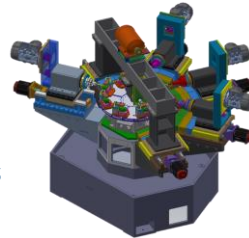
8 station special purpose machines
