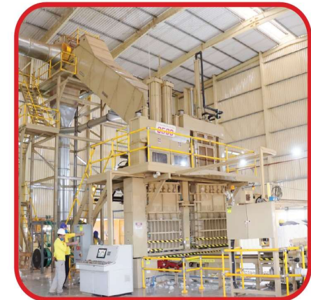
BAJAJ CONTINENTAL 9500 BALE PRESS CAPACITY - 45 & 60 BALES PER HOUR
