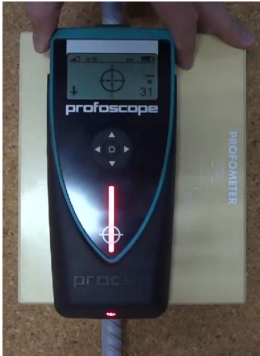
Fig.2.7: Estimating location of rebar
