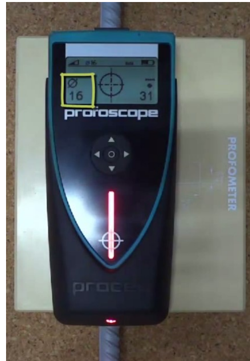
Fig.2.8: Estimating rebar diameter
