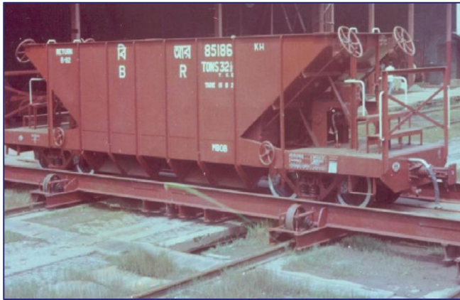
Open hopper side discharge cars for Bangladesh railway
