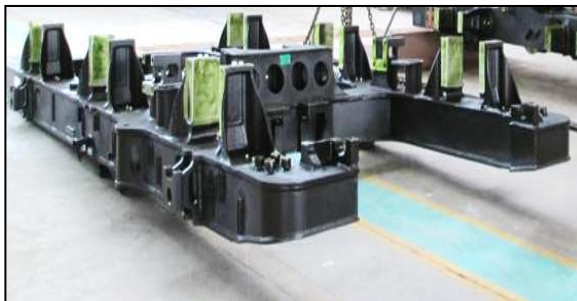
Loco Bogie Frame - Queensland Railways
