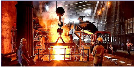
Tapping of Molten Metal from Arc Furnace
