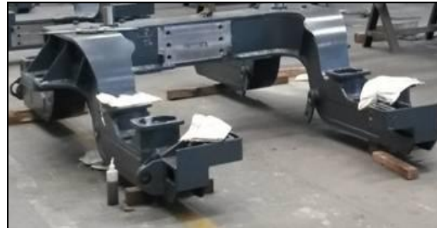
Loco Bogie Frame - Queensland Railways
